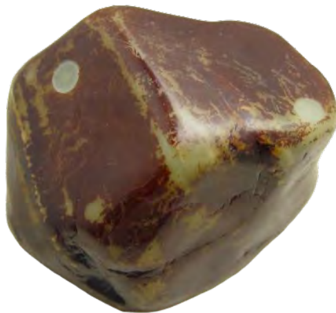
A coloured coating artificially applied to a nephrite boulder, the circled area are where the coating has been removed.
