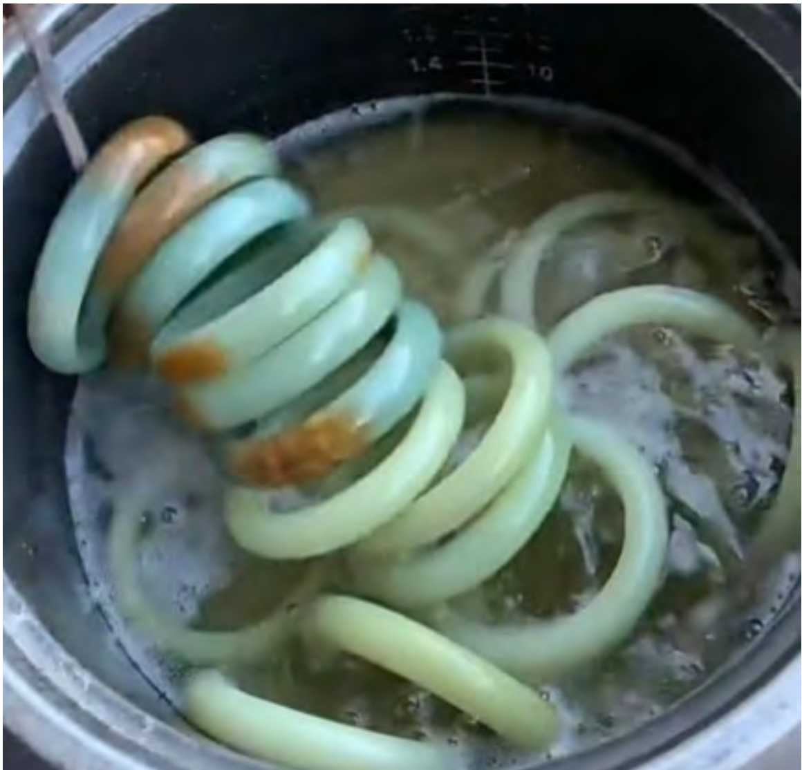
Nephrite bangles are heated, dipped in molten wax, and polished to improve the surface appearance.
