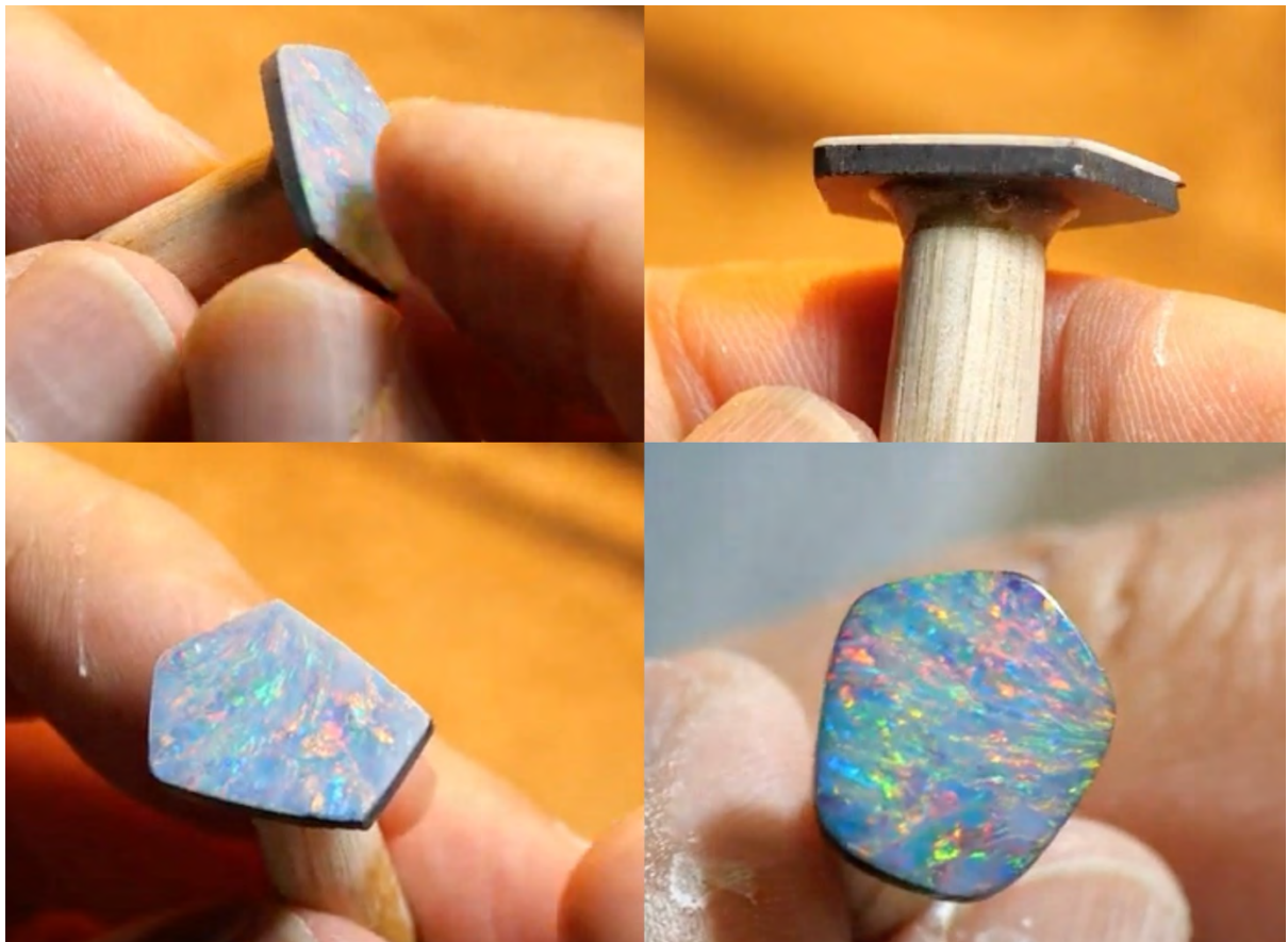
Opal doublet construction (images taken from https://www.youtube.com/watch?v=zrjdeeEeN8 )
