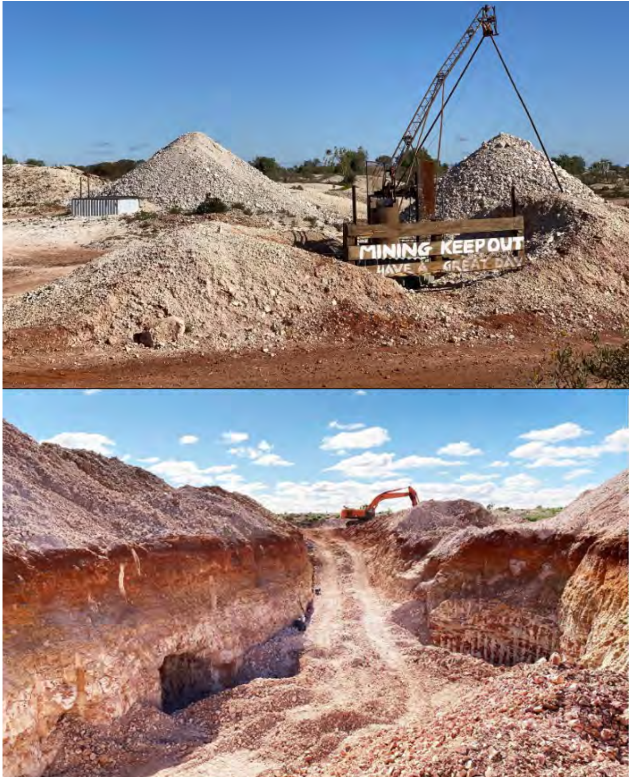
(Top) Shaft with bucket hoist, White Cliffs (image T. S. Coldham – Gemmological Association of Australia) (Bottom) Open cut excavation with old drive exposed, White Cliffs (image T. S. Coldham – Gemmological Association of Australia)
