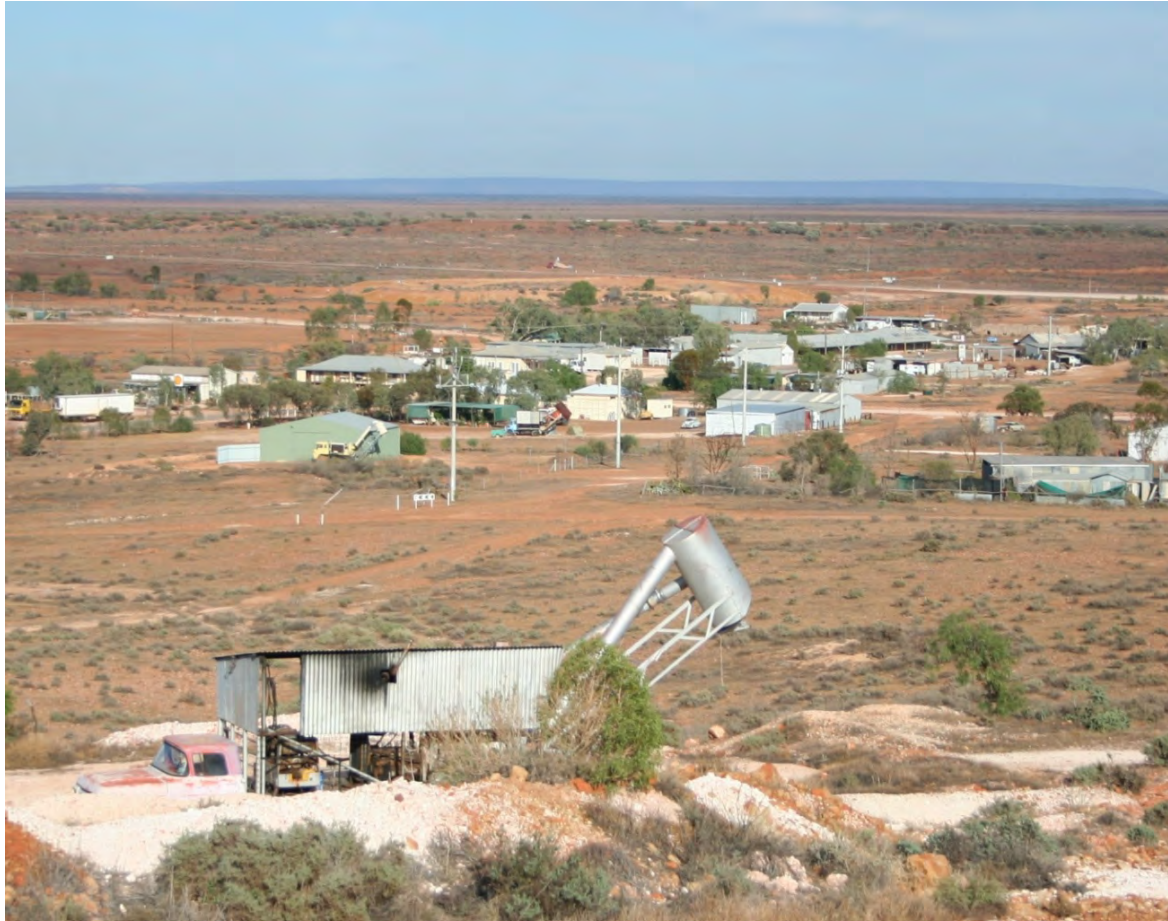
White Cliffs showing shaft with self-loading bucket hoist in foreground (image Anthony Smallwood)
