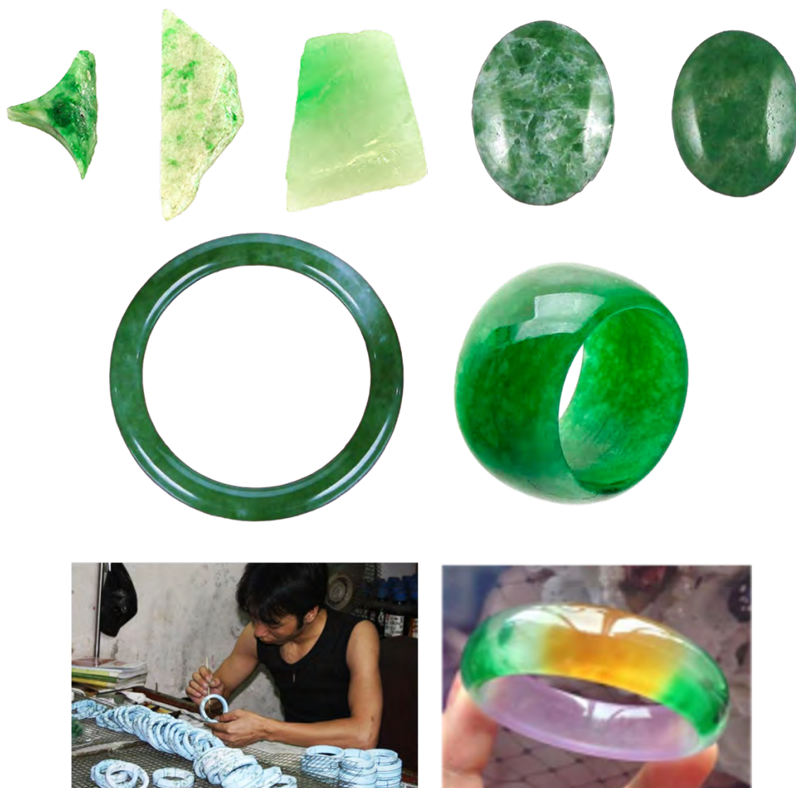
The bleaching, dyeing and impregnating of jadeite jade/fei cui; upper left (left to right) three images show before, during and after bleaching and polymer impregnation (Mayson Kay image) upper right two images bleached (left) and polymer impregnated (right) (Shane McClure image) centre left polymer impregnated bangle (Shane McClure image) centre right polymer impregnated and dyed bangle (Image SSEF) lower left painting bleached bangles (Mayson Kay image) and lower right a bleached, dyed and impregnated bangle (NGTC image).
