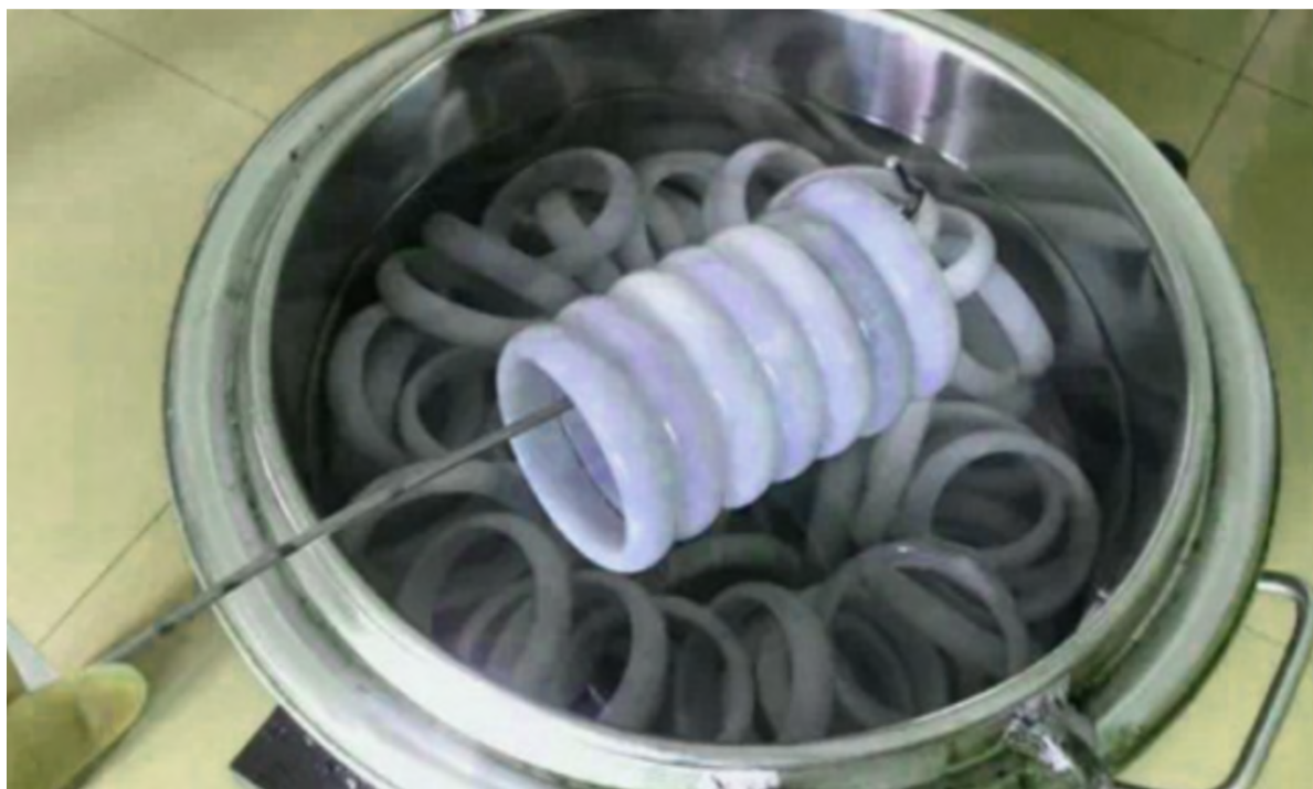
Jadeite jade/fei cui after heating or even unheated is often dipped in liquid wax to improve the surface polish and appearance. Image shows heated Jadeite jade/fei cui in the foreground and immersed in liquid wax in the background.
