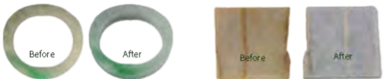
Examples of jadeite jade/fei cui before and after surface bleaching, adapted images from NGTC
