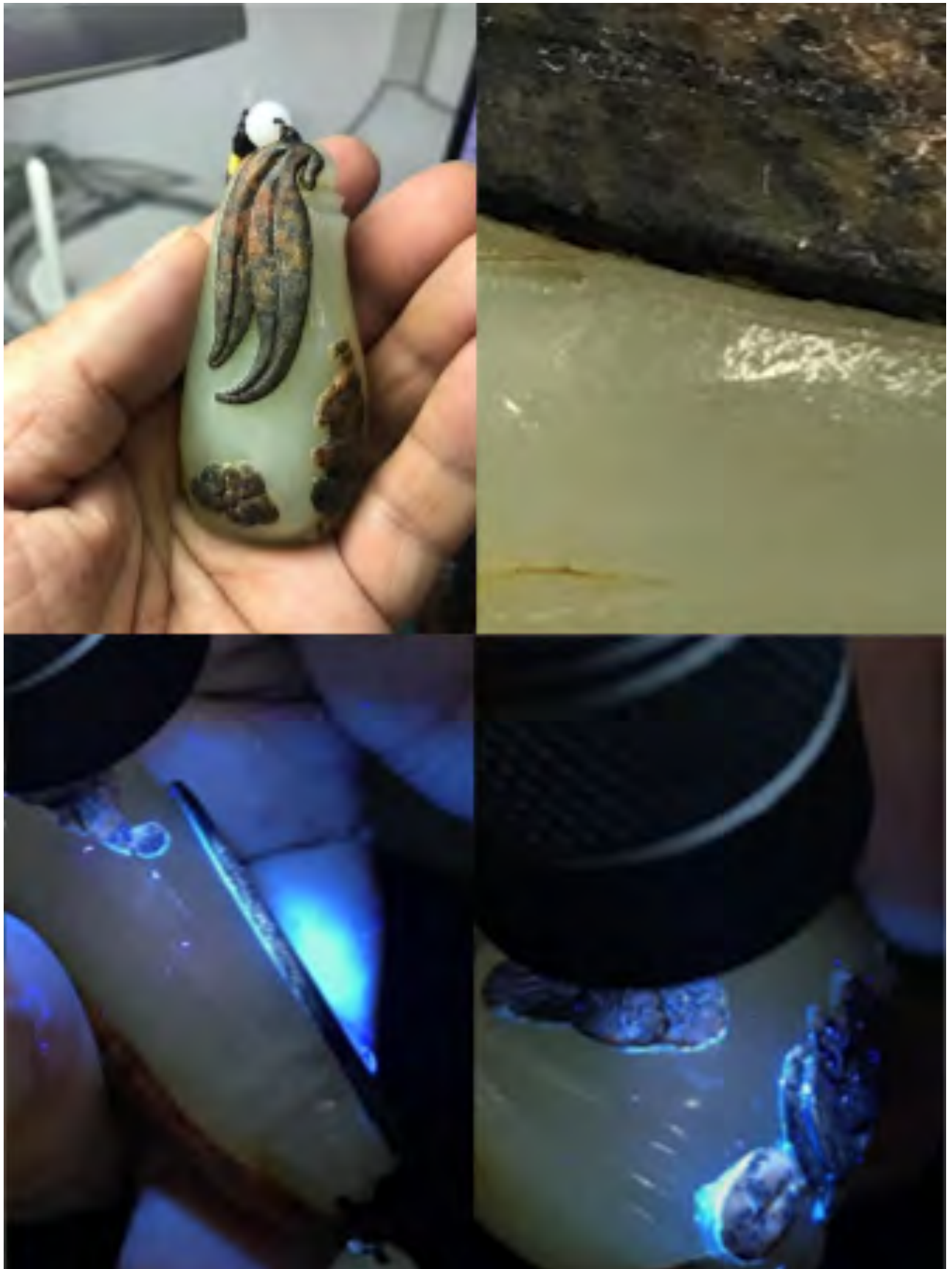
Composite nephrite jade where it can be seen that the brown carvings have been artificially adhered to the base material,
