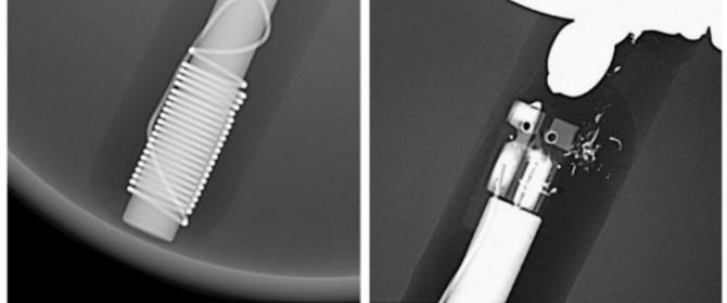
Detail of a coiled wire around one end of a metal caps.ule t (left) and the two contact points at the opposite end (right) seen within an atypical bead cultured pearl.(C. Y. W. Au 2020)
