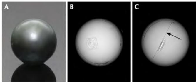
Externally, this specimen with an RFID chip embedded (A) looks no different from bead cultured pearls routinely seen in the market. However, RTX examination revealed a square chip positioned inside a recess within a sawn and reconstructed shell bead (B and C). The arrow in image C indicates the sawn plane (C. Y. W. Au 2020)
