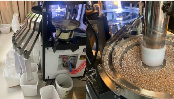
Figure 1An automated cultured pearl sorting instrument in China
